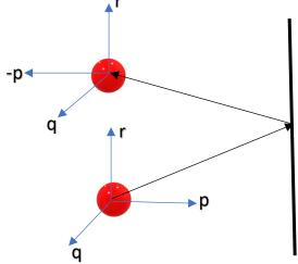
Hence the change in momentum suffered by that molecule during collision is 2mp [m is the mass of the gas molecule]. The other components of velocity do not suffer any change. So, they do not contribute to pressure.
