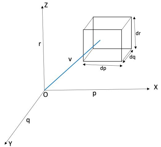
In this diagram a molecule with velocity  $\mathbf{v}^{\mathbf{v}}$  and velocity components p,q,r is represented by a point whose coordinates are (p,q,r). This point is called velocity point.
